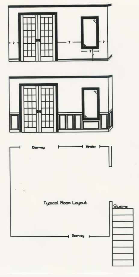
Under the stair wainscoting. Sketch on paper your basic situation with any measurements that pertain to the wainscoted area.
