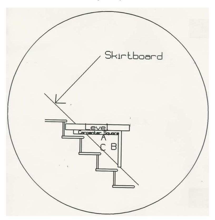
Place a carpenters square on one of the treads as shown. Draw on paper the triangle showing the wall above the stringer & write down the corresponding measurements for "A", "B" and "C".
